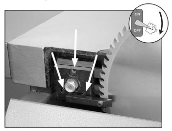
Figure 39. Set screws for adjusting riving knife.
